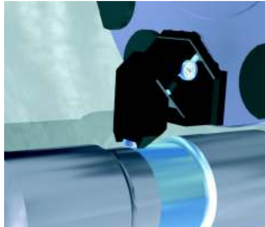
Machining a train axle with an EG45-40M tool.
